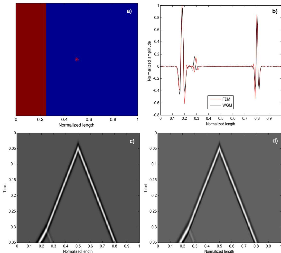
**Figure 4:** (a) Velocity profile (red region is a faster medium) and source position; (b) Snapshot for amplitude comparison at time  $t=0.35s$  for example 2; (c) Seismogram obtained using WGM; (d) Seismogram obtained using FDM with noticeable numerical dispersion.
